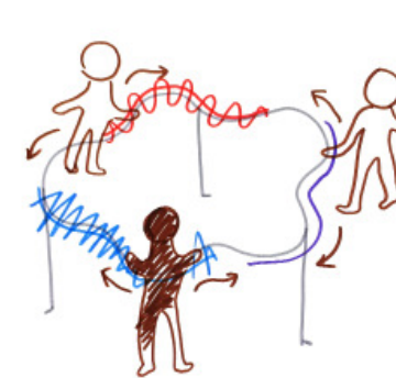
When elderly exercise or walk along the device, the light moves in a rhythm. When there are multiple rhythms the light combines these so they can interact with each other.
