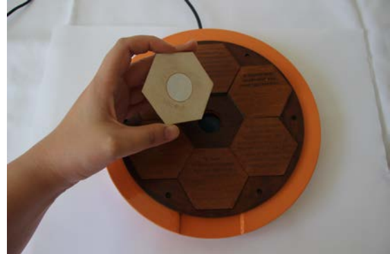
The middle part contains an RFID chip making the goals linked to a particular student or group.
