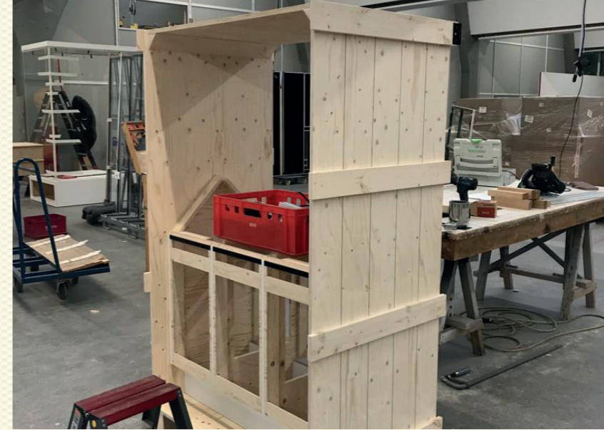
Figure 51. art transport case put together before spray painting (own photograph)
